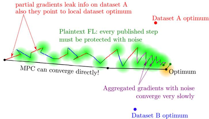
**Fig. 4.** Compared convergence: MPC versus plaintext-aggregation FL.
