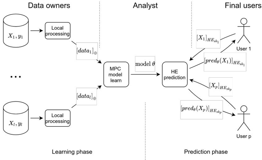
**Fig. 1.** GenoPPML architecture. Private datasets are processed locally for dimensionality reduction and outputs are secret shared for model training in MPC. The computed model is then used for prediction on users’ data encrypted via an FHE scheme. Users receive and decrypt the computed encrypted predictions.
