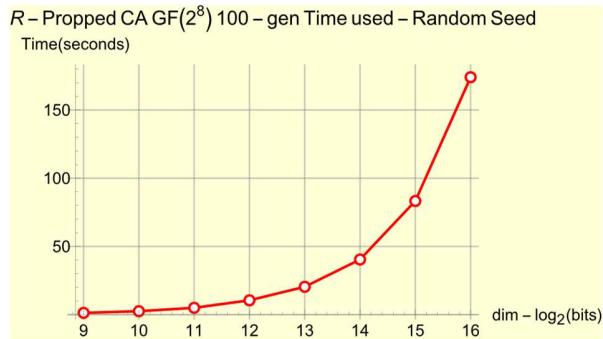
**Table 12.** The computation time of 100-generation runs of a Mathematica interpreted code. The optimal dimension for concrete applications should be chosen as high as the restrictions allow.
