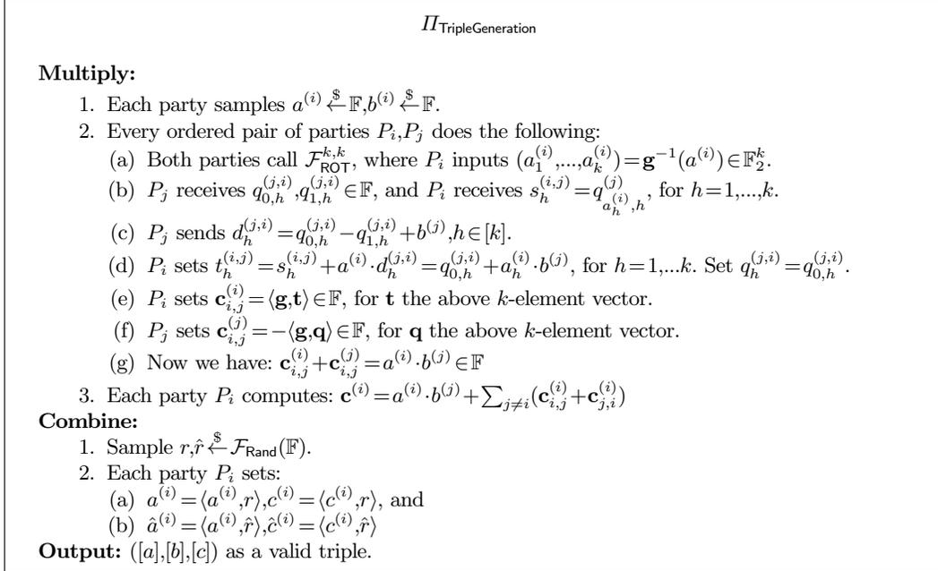
**Fig. 19.** Protocol for Triple Generation adjusted for passive security from MASCOT [KOS16].
