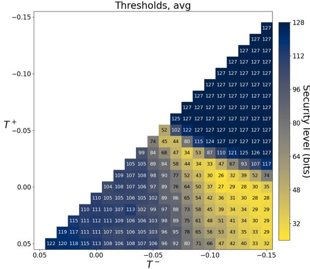
Fig. 7: Average performance of our attack on 2048 plaintexts, averaged from 2048 traces each, with varying values of  $T^+$  and  $T^-$ . Note that the attack performs at its worst for low  $T^+$ ,  $T^-$ —this is because we mistakenly classify every measurement as a positive in this configuration, and thus our attack can extract no constraints.
