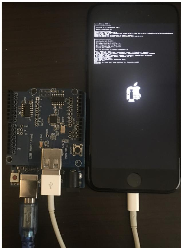
Fig. 2: Arduino with `MAX3421E` USB host shield connected to our test iPhone 7. The Arduino is a USB proxy between the host and device and generates correct partial requests when necessary. This setup successfully addresses `checkm8`’s reliability issues. This iPhone is running `pon-goOS`, briefly discussed in Section IV-B.
