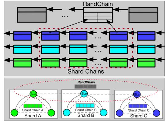
Fig. 3. Overview on the RandChain Protocol Design. The upper shows on the contraction of chains, and the lower part shows the connections among participating nodes.
