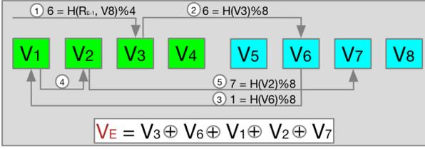
Fig. 2. Example of the *Cast* Phase of RandGene Protocol, where  $k = 8$ .
