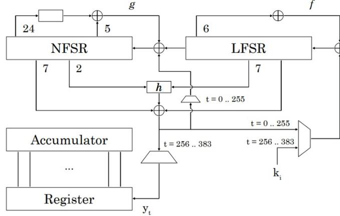
**Fig. 1.** Overview of the Initialization of Grain-128AEAD
