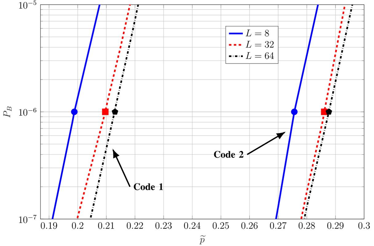
Fig. 4. Block-error probability of  $\mathcal{C}$  over a BSC with crossover probabilities  $\tilde{p}$  for Codes 1 and 2 of length 1024 and 2048 bits, respectively, with sequential decoders and corresponding  $\bar{p}_c$  values represented by a circle for list size  $L = 8$ , square for  $L = 32$ , and pentagon for  $L = 64$ .
