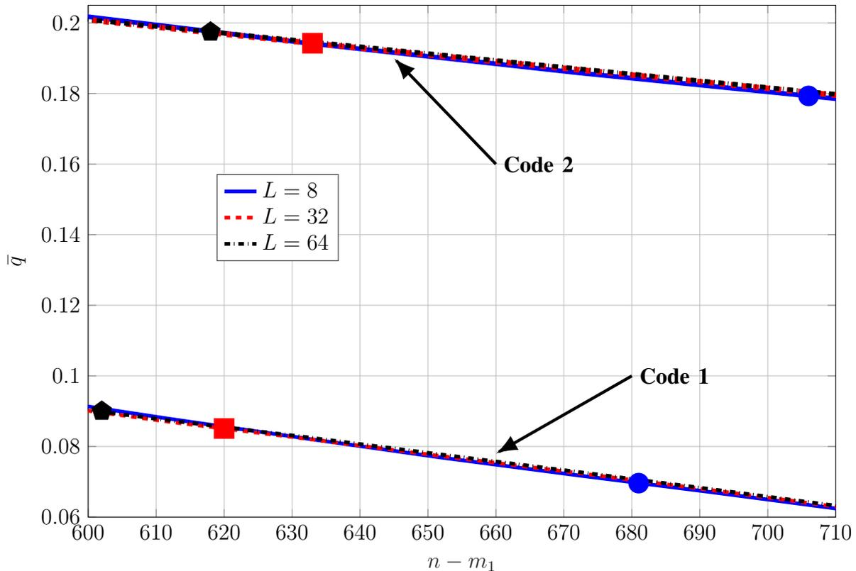
Fig. 5. Average distortion  $\bar{q}$  with respect to  $n - m_1$  for Codes 1 and 2 with sequential decoders and corresponding  $E[q]$  values represented by a circle for list size  $L = 8$ , square for  $L = 32$ , and pentagon for  $L = 64$ .
