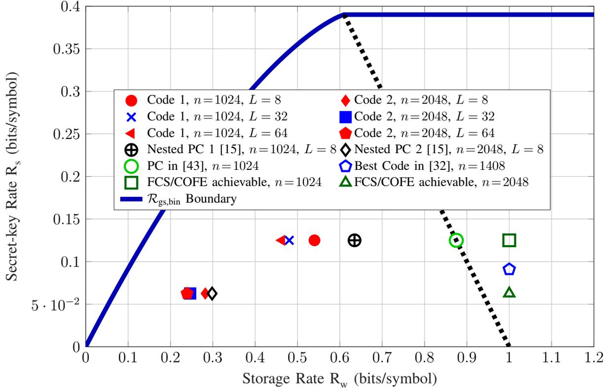
Fig. 6. Storage-key rates for key generation with crossover probability  $p_A = 0.15$ . The block-error probability satisfies  $P_B \leq 10^{-6}$  and the key length is 128 bits for all code points. The dashed line represents  $R_w + R_s = H(X) = 1$  bit/symbol. All codes with  $R_w = 1$  bit/symbol are ECCs. The PC on the dashed line is a syndrome-coding construction.
