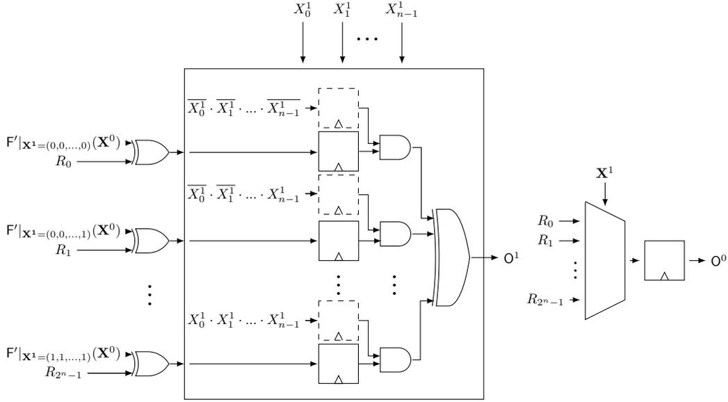
Figure 4: General GHPC<sub>LL</sub> design with reduced latency.
