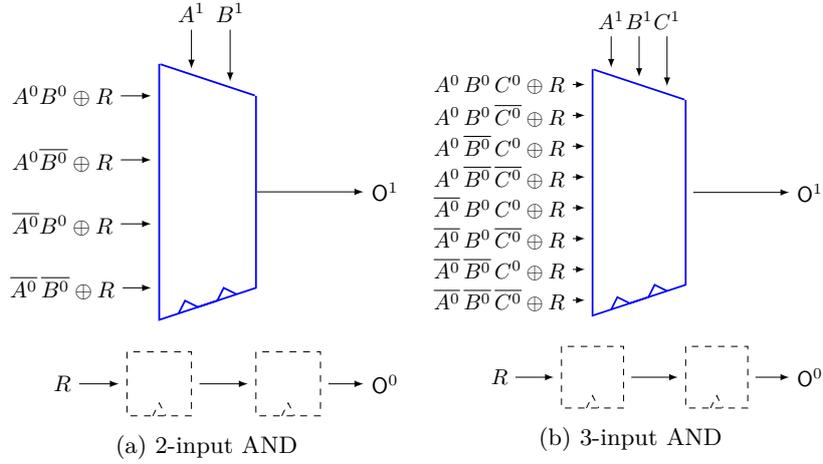
Figure 3: Examples for first-order PINI-secure GHPC constructions.
