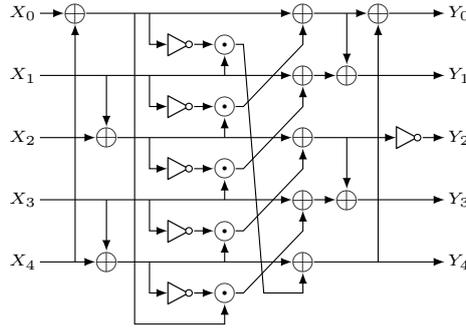
Figure 4: Bitsliced implementation of the substitution layer
