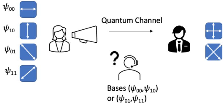
Fig. 1: An illustration of the BB84 protocol for the qubit transmission for the key exchange. The sender Alice (left) transmits the qubits in one of the four states, e.g.,  $\psi_{00}$ , while the receiver Bob (right) uses either of the two bases to make measurements on the received qubits.
