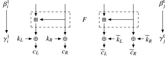
**Fig. 5.** A toy example of key recovery where the key-recovery part  $F$  only contains a modular addition.
