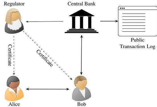
Figure 1: **Platypus System model.** Platypus consists of a central bank that is responsible for transaction validation, a regulator that issues certificates to clients and receives transaction information relevant for compliance with regulatory rules, as well as clients that participate in the system. The central bank also publishes a log of all transactions.
