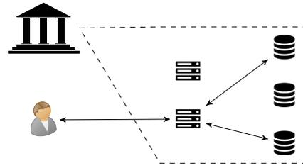
Figure 3: **Sharding Potential in Platypus.** The central bank can shard both computation and the storage of serial numbers internally. A client can connect to an arbitrary compute node (e.g. through a load balancer) which validates transactions independently from other compute nodes. The compute node then uses a two-phase commit to check and update serial numbers in the database shards corresponding to the serial numbers of the sender and recipient.
