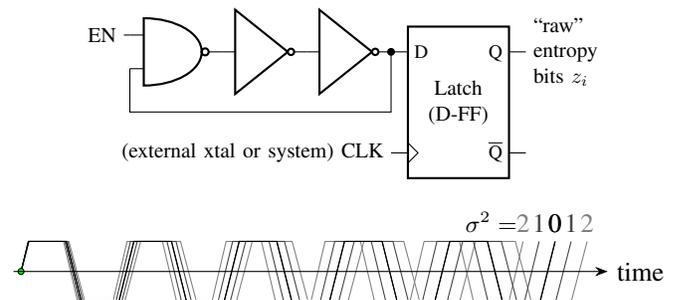
Fig. 1. A ring oscillator consists of an odd (here  $N = 3$ ) number of inverters connected into a free-running loop. The output is sampled using an independent reference clock, such as a crystal oscillator. Transition times are affected by jitter (largely from Johnson-Nyquist thermal noise), whose accumulation causes samples to become increasingly unpredictable.
