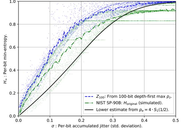
Fig. 4. Min-entropy from distribution of  $Z_{100}$  with depth-first  $z$  selection, NIST SP 800-90B estimates, and our  $p_e$  bit-prediction lower bound. Experimental data is represented as a scatter plot, with a line at the average.
