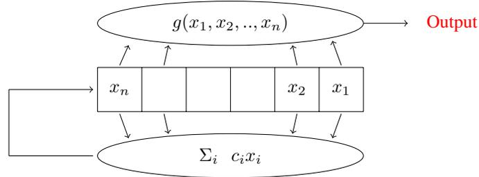
Fig. 1. Stream generator with with 1 LFSR
