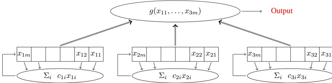
Fig. 2. Stream generator with 3 LFSRs
