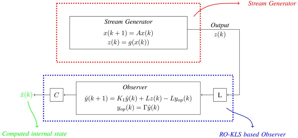
Fig. 4. Dynamic Observer for Stream generator using RO-KLS
