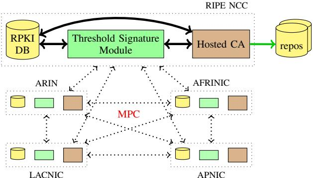
Fig. 2. Distributed RPKI architecture
