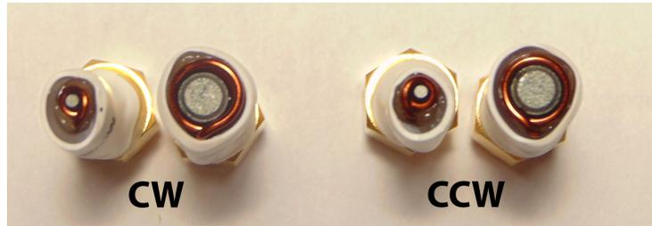
Fig. 2: Showing the wire wrapping direction around the injection tip (coil).
