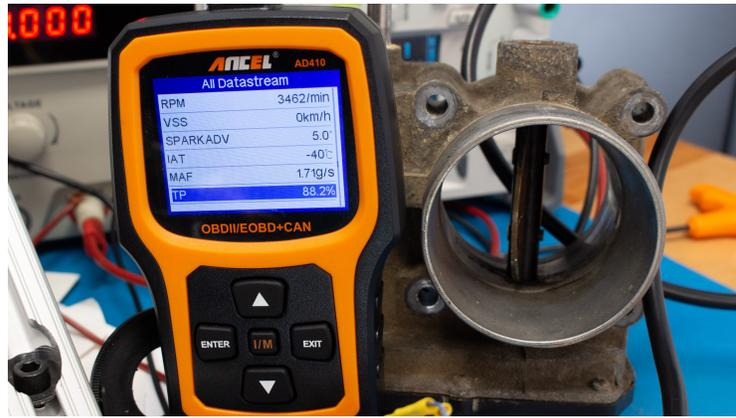
Fig. 8: The ECU after an EMFI based fault caused some error where the throttle is commanded to become fully open.
