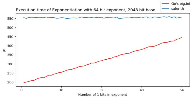
Figure 1: Execution time of exponentiation (Exp), averaged over 400 runs, with an increasing number of set bits. For `big.Int`, execution time is clearly correlated with this value. For `Nat`, we observe no such correlation.
