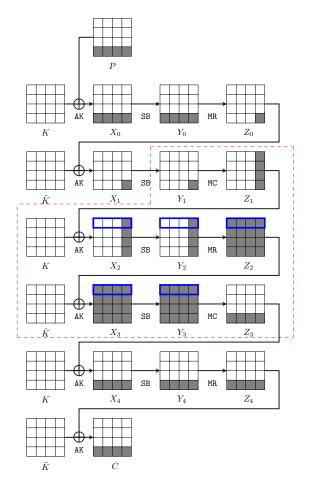
Fig. 16: Classic collision attack on 5-round Saturnin
