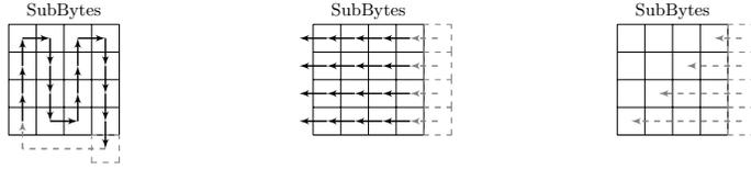
Fig. 6: Three examples of diffusion patterns using the changing of the guards technique. Additional cells are outlined by dashed gray lines. The third example chains all cells in a row.
