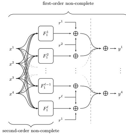
Fig. 5: Sharing of the cubic function  $F$  (or  $G$ ). The Boolean functions  $F_1^1, \dots, F_1^\ell$  are the shares of the first layer  $\bar{F}_1$  (or  $\bar{G}_1$ ). The gray dashed line denotes a register stage.
