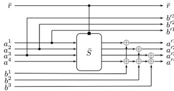
Fig. 2: Changing of the guards method with four shares where the shared S-box  $\bar{S}$  uses the randomness  $\bar{r}$ .
