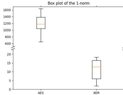
Fig. 11: Box plot of the 1-norm of the Walsh-Hadamard transform of the glitch functions for the masked AES and the XOR, for different probe positions, times, input delays and initial states.
