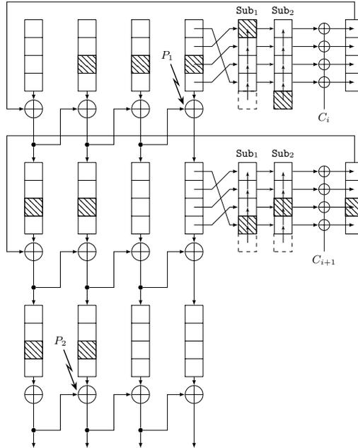
Fig. 9: Activity pattern of a trail with non-zero correlation through two rounds of the second-order masked key schedule of AES caused by two probes. Hatched cells correspond to active cells. The lightning signs denote the two probes.
