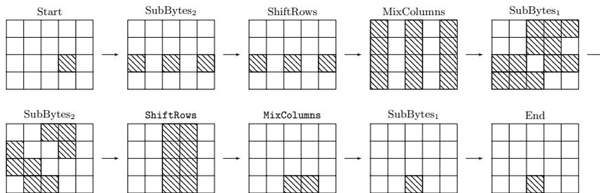
Fig. 12: An optimal trail (for two probes) with non-zero correlation through the second-order masked AES. The hatched cells denote active cells of the output of the operation.
