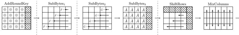
Fig. 4: One round of the masked AES. The locations of the registers are indicated by dashed lines. The nonlinear operations require an additional register stage, which is not shown on the figure. Hatched cells remain unchanged through the operation.
