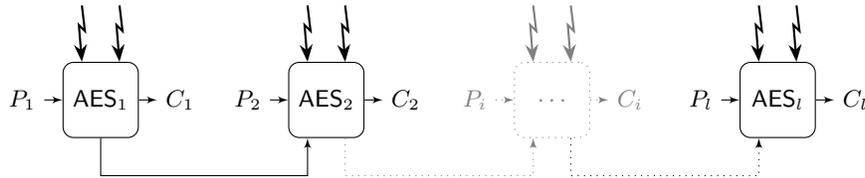
Fig. 8: Illustration of the  $l$ -block 2-threshold probing model.
