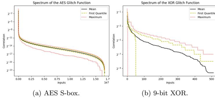
Fig. 10: Sorted absolute Walsh-spectrum of glitch functions for the AES S-box and the 9-bit XOR for different probe positions, times, inputs delays, and initial states.
