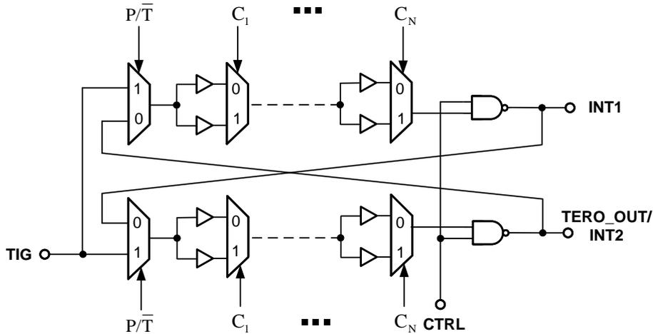
Figure 1: Proposed Architecture of a dual-mode TERO Cell.
