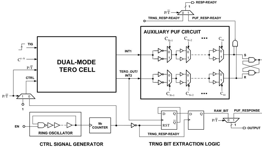
Figure 2: Unified PUF-TRNG Architecture with dual mode operability.
