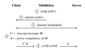
Figure 1: Structure of our ZKMB protocol. The client convinces the middlebox that the message *M* is policy-compliant without revealing it. The handshake and encryption algorithms are part of the underlying secure channel (such as TLS). Transcripts and secrets generated in the handshake may be inputs to the proving and verification steps.
