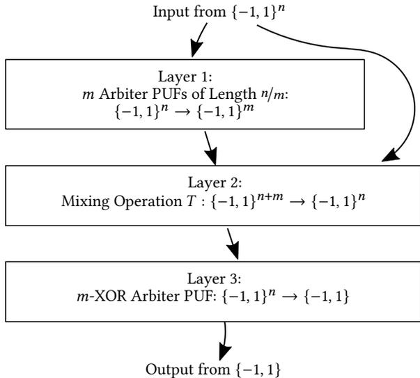
**Figure 1: The LP-PUF design, parameterized by the challenge length  $n$  and the additional security parameter  $m$ .**
