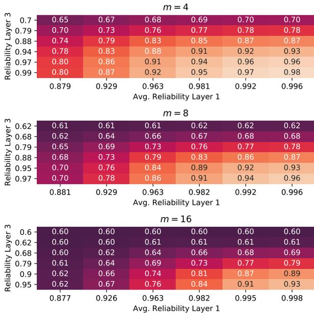
**Figure 4: Simulated reliability of the 64-bit LP-PUFs depending on reliabilities of the building blocks.**
