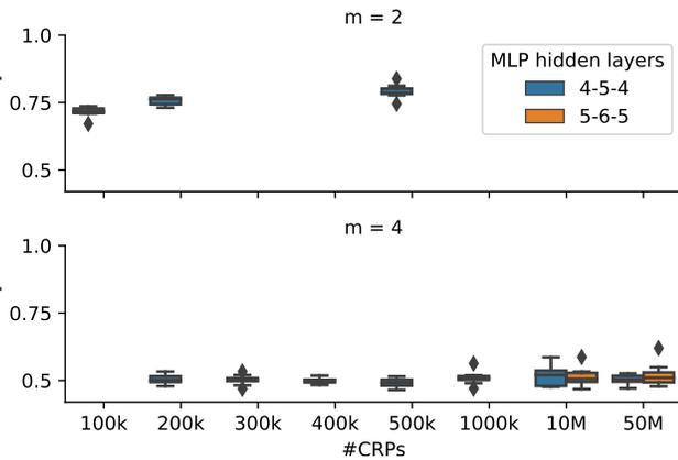
**Figure 7: Prediction accuracy of the MLP attack by Wisiol et al. [23] run on 64-bit  $m$ -LP-PUF. The neural network, training parameters, and – perhaps most importantly – the features were not modified from the original version. Due to the attacker-unknown challenge to Layer 3 of the LP-PUF, it is unclear how the attacker should adjust the features.**
