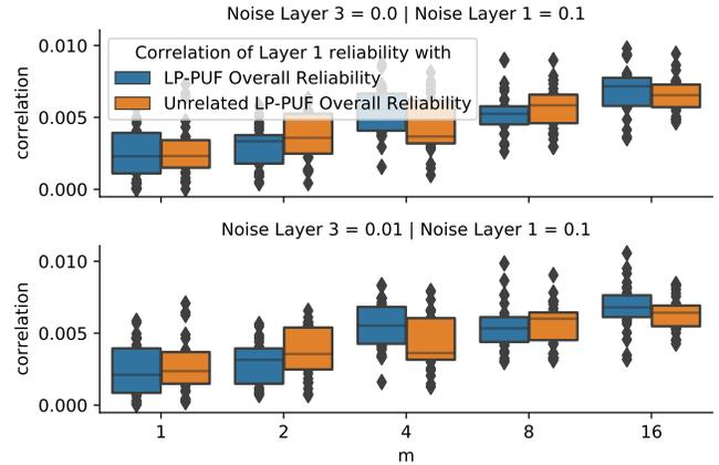
**Figure 5: The correlation of the attacker-observable overall reliability of a given  $n = 64$  challenge bit LP-PUF with the reliability of Layer 1. To account for all response bits of Layer 1, the maximum correlation in each instance is taken. If a large correlation of Layer 1 reliability and LP-PUF reliability can be established, an attacker could attempt a reliability-based modeling attack on Layer 1.**
