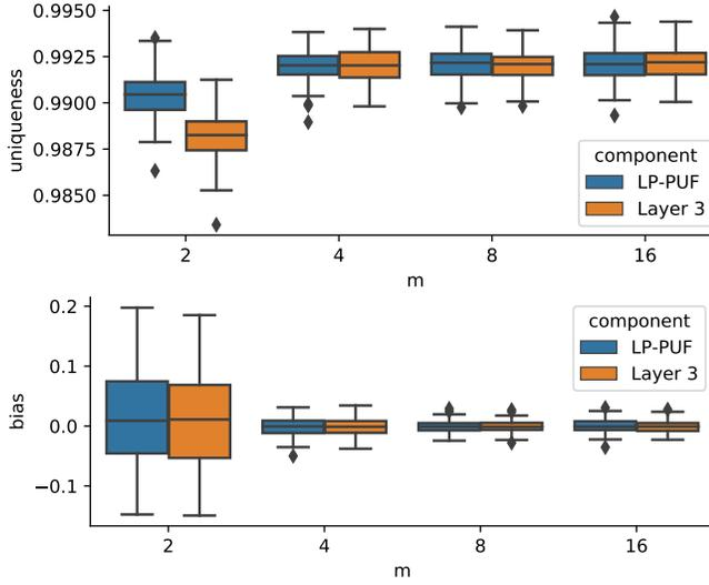
**Figure 2: Uniqueness and bias of the proposed LP-PUF, measured in noise-free simulations and for  $n = 64$  challenge bits across different values of the  $m$  parameter. For comparison, the corresponding metrics are also shown for Layer 3 of the LP-PUF, which consists of a traditional  $n$ -bit  $m$ -XOR Arbiter PUF.**
