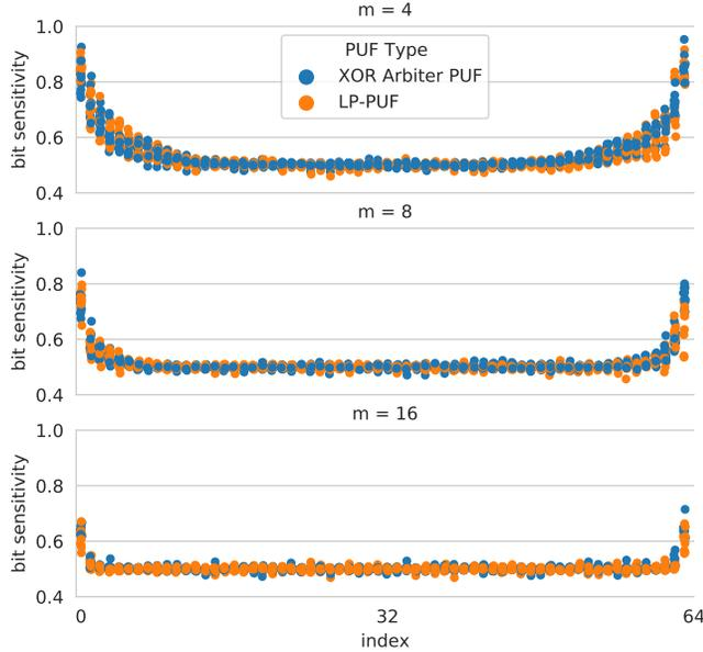
**Figure 3: Bit sensitivity values for the LP-PUF and XOR Arbiter PUF for both 64-bit challenges. Values of  $1/2$  are ideal.**
