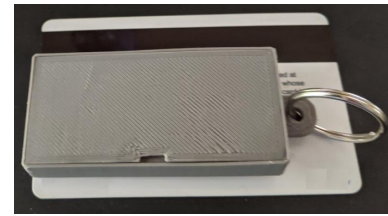
Figure 2: Entire device enclosed in the preliminary 3D printed case prototype, in preparation for deployment. The longest dimension is 1 cm longer than the board to accommodate the rechargeable battery.
