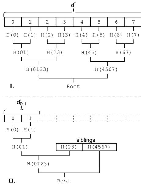
Fig. 11: **I.** The calculation of root in *hash* phase. **II.** The verification of the root in *resubmit* phase.  $H(k)$  denotes the digest of element  $k$ .  $H(kl)$  denotes the result of  $H(H(k) | H(l))$
