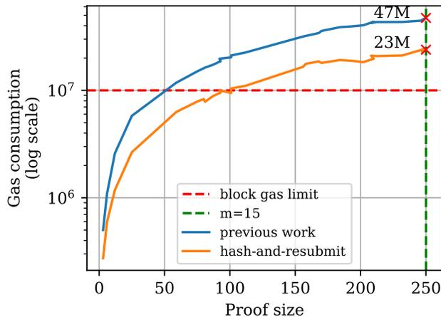
Fig. 5: Gas consumption of our NIPoPoWs verifier enhanced with hash-and-resubmit compared to previous work (lower is better) using a secure value of  $m$ . Gas consumption is decreased by approximately 50%.
