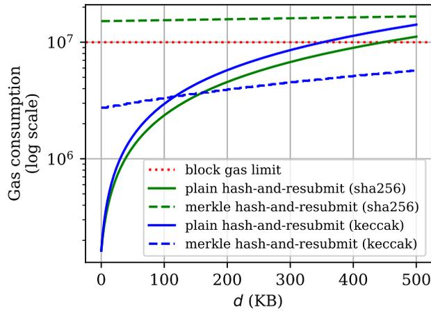
Fig. 12: Trade-offs between *hash-and-resubmit* variations. In the vertical axis the gas consumption is displayed. In the horizontal axis the size of *d*. The size of *d*<sub>0</sub> is 10KB bytes, and the hash functions we use are the pre-compiled *sha256* and *keccak*.
