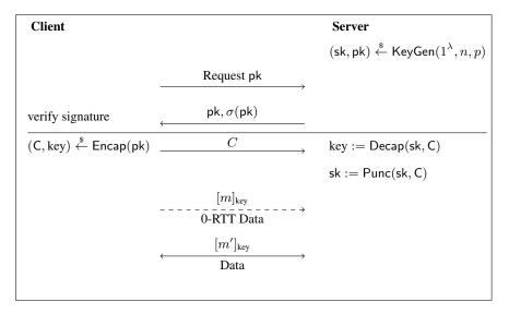
**Fig. 2.** Simplified version of the implemented handshake protocol.  $\sigma(\cdot)$  denotes a signature, computed with the server's long-lived signing key. If the server's pk is known, only the part below the horizontal divider is executed
