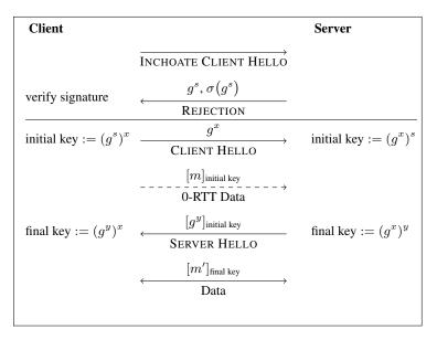
Fig. 1. Simplified QUIC handshake protocol.  $\sigma(\cdot)$  denotes a signature, computed with the server's long-lived signing key. If the server's  $g^s$  is known, only the part below the horizontal divider is executed.
