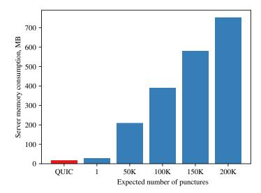
**Fig. 6.** Server memory consumption for different expected number n of punctures over the lifetime of the public key and fixed bound on the failure probability p=0.001 with point compression disabled. The linear increase of memory consumption in n is due to the larger secret key array size m required to guarantee the chosen bound on the failure probability. The memory consumption of the QUIC server is shown for reference.
