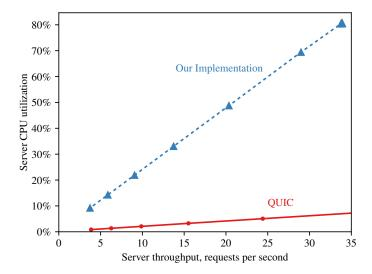
**Fig. 5.** Server CPU utilization for a given throughput. The measurement of our implementation is compared with the original QUIC implementation. Note that we plot in the range from 0 to 35 requests per second, which encloses the throughput limit of our implementation.
