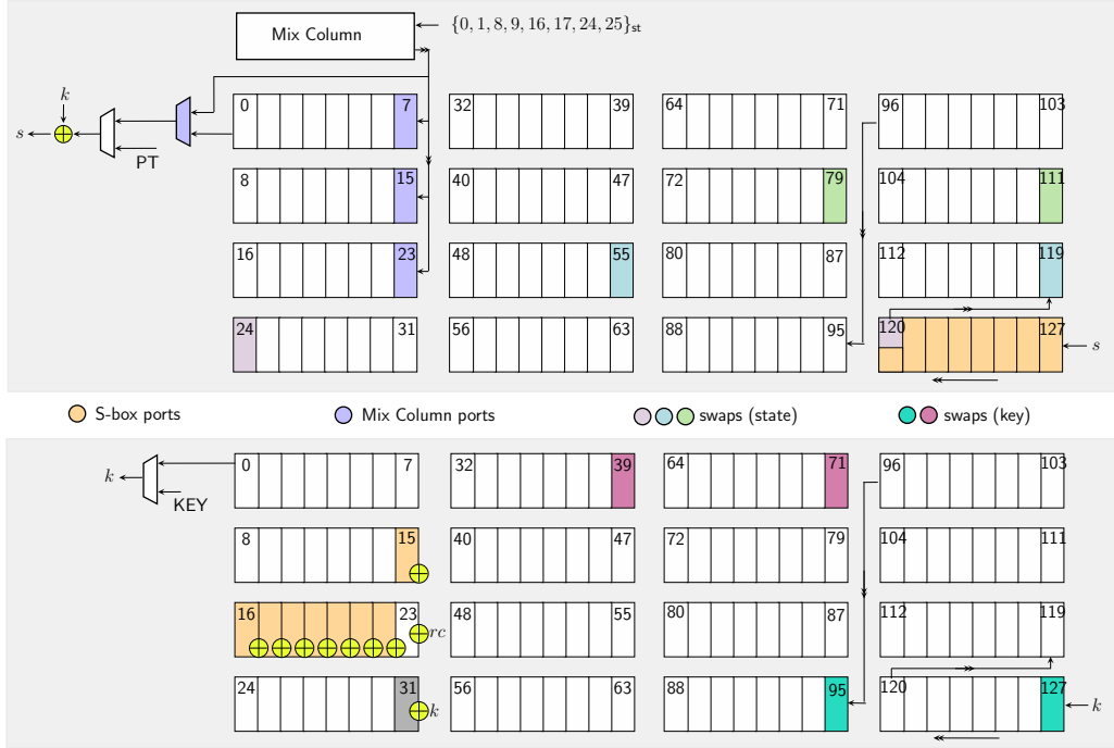
Figure 2: The state (above) and key (below) pipelines of AES-128 encryption with colored scan flip-flops.
