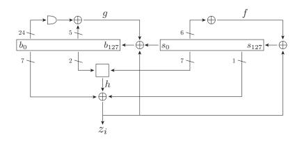
Fig. 5. Structure of Grain-128AEAD
