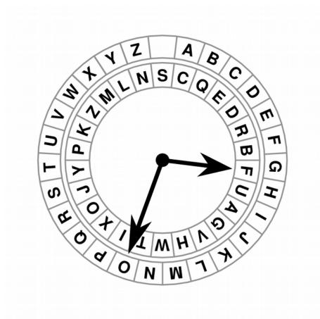
Figure 2. Schematic sketch of the Wadsworth cipher disk. The mixed ciphertext alphabet is taken from the example found in the NSA file (1951). The rings of characters rotate counterclockwise under a fixed pointer by the same number of steps, but not through the same angle.
