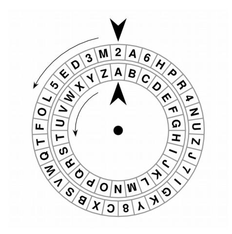
Figure 3. Schematic sketch of Urkryptografen. The mixed alphabet shown here is from the photograph found in Faurholt's article (2003). The rings of characters rotate counterclockwise under a fixed pointer by the same number of steps, but not through the same angle.
