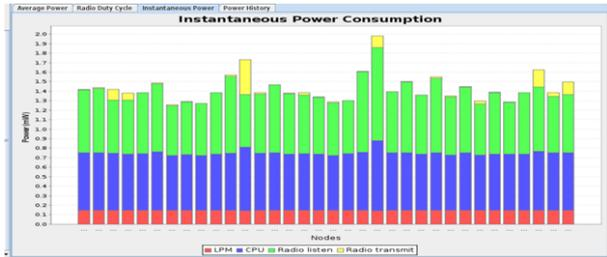
Figure 23: Sinkhole attack average power consumption
