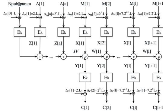
Fig. 2. COLM authenticated encryption mode of operation [7]
