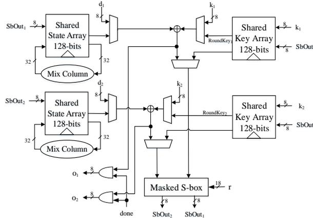
Fig. 11. Proposed Hardware architectures for DOM protected AES-128
