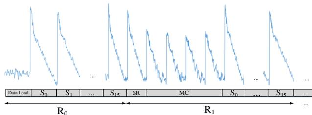
Fig. 6. A measured power trace for the initial and first round of unprotected AES
