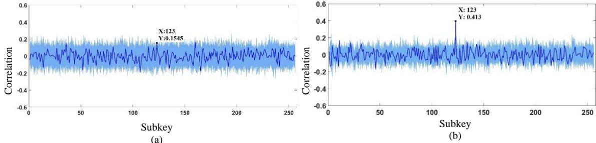
Fig. 13. CPA attack results on protected COLM using ZV model with 1,080 traces (a) the first-order attack and (b) the second-order attack
