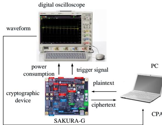
Fig. 5. Setup for capturing trace with the SAKURA-G
