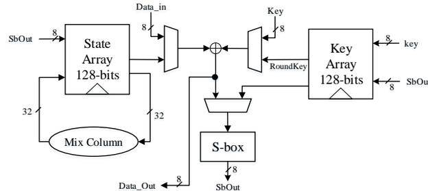
Fig. 4. AES architecture for the attack against COLM [24]
