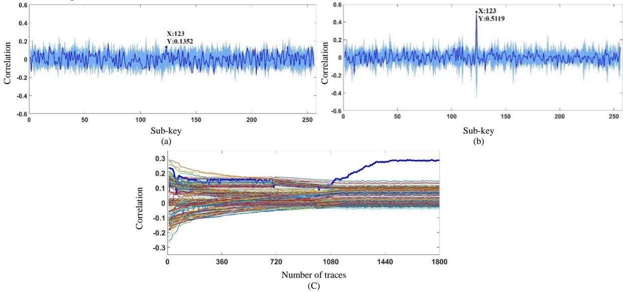
Fig. 7. CPA attack results on unprotected COLM using 1,800 measurements ( $K'_0$  is obtained) at time 1.67  $\mu$ s (a) HD, (b) ZV model (c) over the traces number
