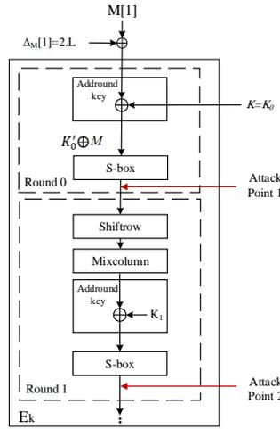
Fig. 3. Attack procedure on the initial and the first round of AES in unprotected COLM
