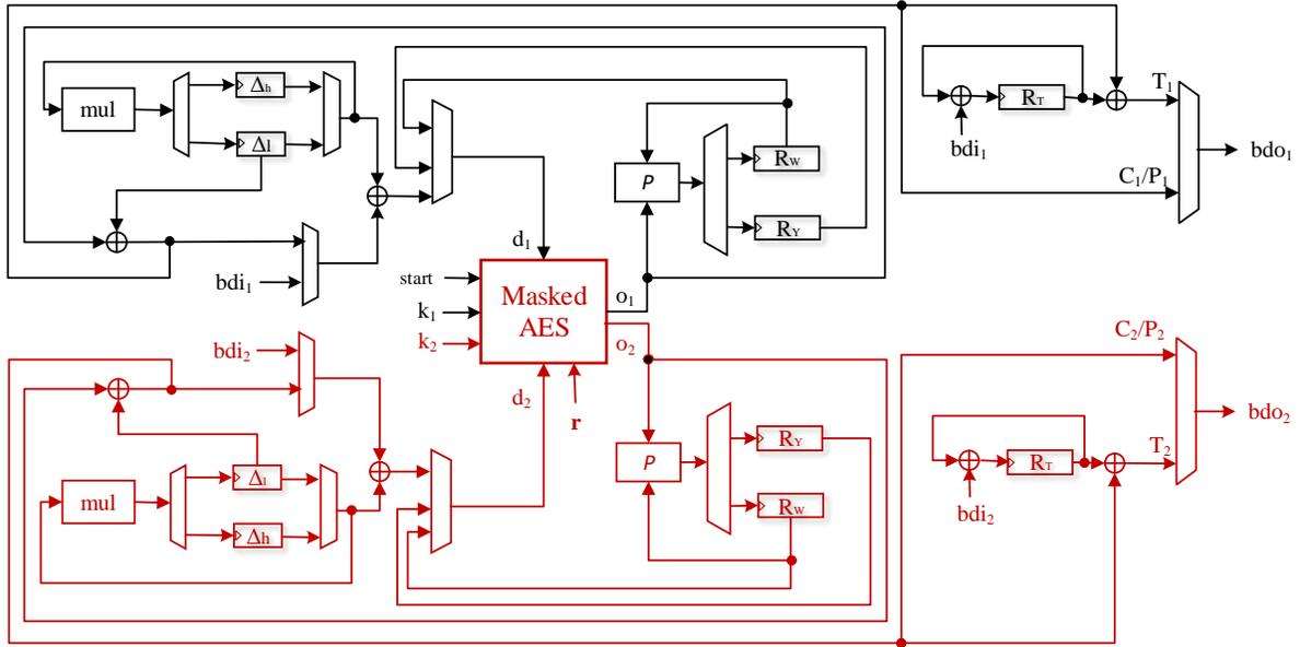
Fig. 9. The proposed 8-bit hardware architecture for protected COLM
