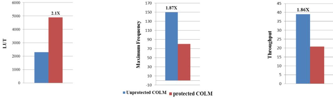
Fig. 12. Area (in LUTs), maximum frequency and throughput comparison ratios of unprotected and protected COLM
