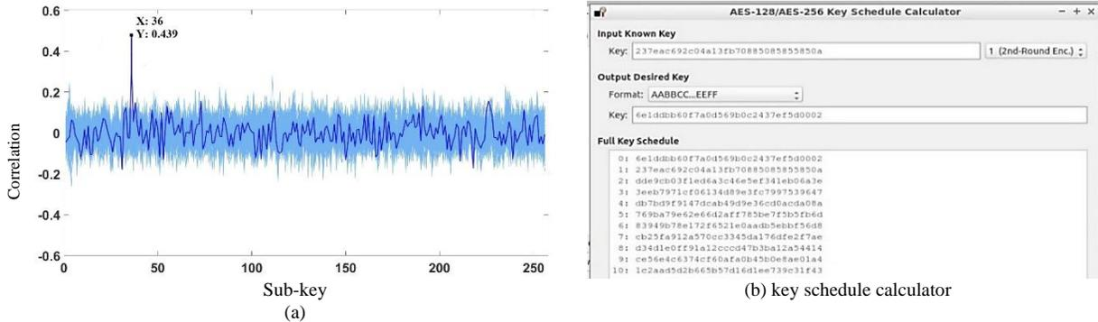
Fig. 8. CPA attack results on unprotected COLM (a) first round key and (b) encryption key
