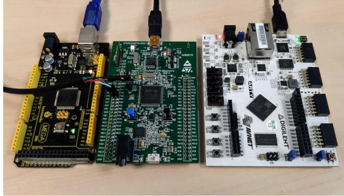
**Figure 2:** A “family portrait” of the development boards used in this work. From left: An Arduino compatible ATmega2560 board (AVR Architecture), STM32F407-Discovery (Cortex M4, ARMv7-M Architecture), and Arty7-35T XC7A35T (An Artix-7 FPGA used to run our RISC-V RV32I+ ISA core).
