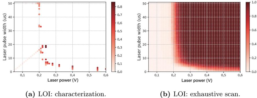
**Fig. 5.** LOI distribution with different fault injection settings.
