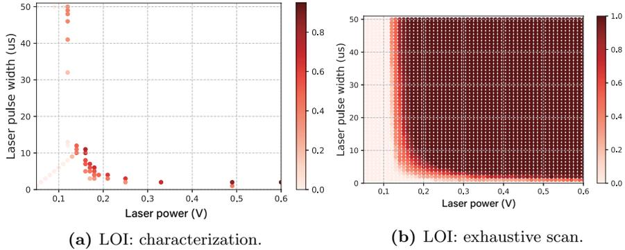
**Fig. 10.** LOI distribution with different fault injection settings.
