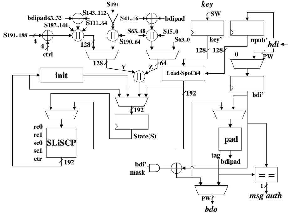
Fig. 5. Block diagram for SpoC-64.
