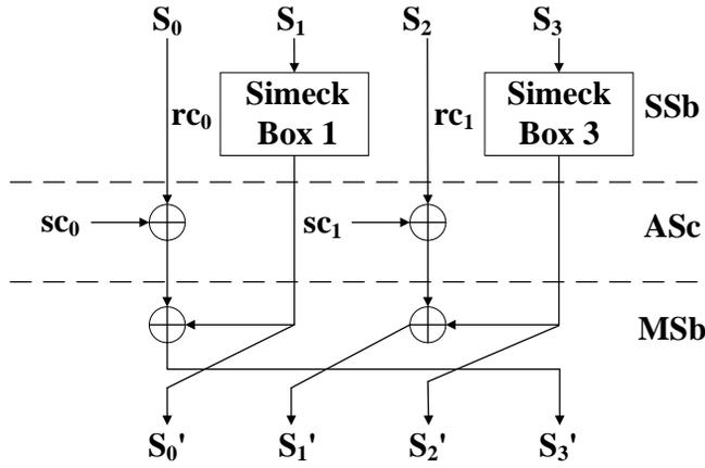
Fig. 3. sLiSCP permutation. Bus widths are 48 bits.
