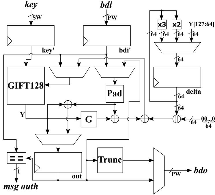
Fig. 10. Block diagram for GIFT-COFB. Bus widths are 128 bits unless indicated.
