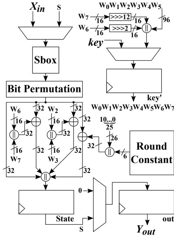
**Fig. 8.** Block diagram for GIFT-128 round function. Bus widths are 128 bits unless indicated.
