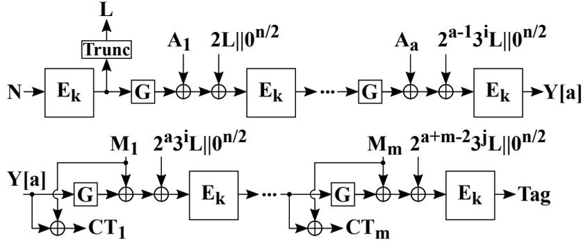
Fig. 9. GIFT-COFB encryption construction.
