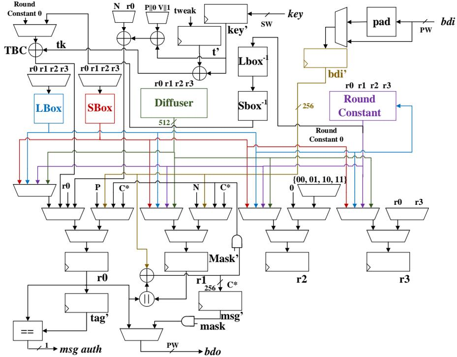
Fig. 7. Block diagram for Spook[128;512;su]. Bus widths are 128 bits unless indicated.
