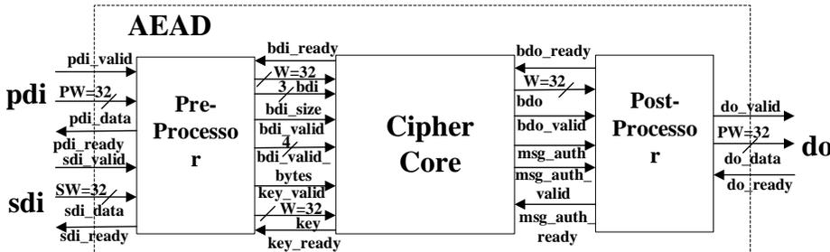
Fig. 1. Instantiation of CipherCore inside AEAD, together with modules and signals from CAESAR HW Developer’s Package.
