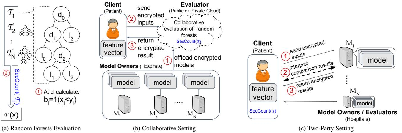
Fig. 1: System models for collaborative evaluation of random forests  $\mathcal{F}$ , consisting of  $N$  decision trees: Each decision tree  $\mathcal{T}_i$  with a depth of  $\delta$  contains  $m$  decision nodes  $d_i \in \mathcal{D}$ , and  $(m + 1)$  leaf nodes  $l_k \in \mathcal{L}$ . Each leaf node contains a classification value  $v_k \in V$ .
