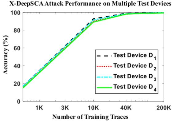
**Figure 6: Attack Accuracy on the test devices ( $D_{1-4}$ ) with the DNN model trained with varying number of training traces gathered from the 4 training devices, where each of them ( $TR_{1-4}$ ) contributed equally .**
