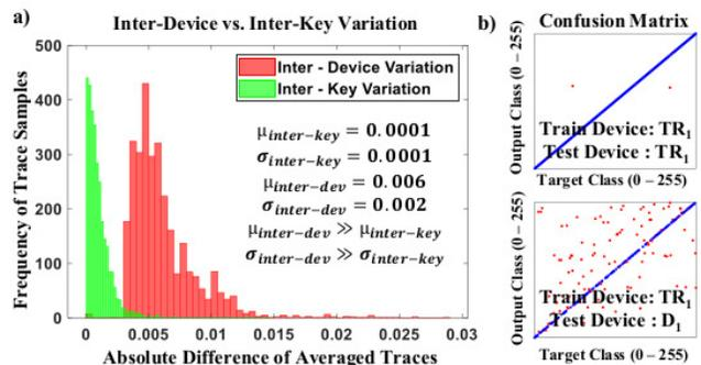
Figure 1: (a) Histogram plot showing that the mean of device-to-device variations of the power traces is significantly higher than the mean of key-to-key (class) variations for one device. (b) Training with one device ( $TR_1$ ), the 256-class DNN is able to classify unseen test traces from the same device ( $TR_1$ ) accurately as seen from the confusion matrix, while it does not generalize for other devices and misclassifies many test traces from a different device ( $D_1$ ).
