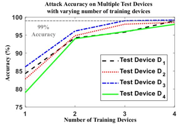
**Figure 8: Effect of augmenting traces from Multiple Devices during training: As the number of devices is increased, the DNN model generalizes well to new devices ( $D_{1-4}$ ) and hence the accuracy improves and reaches 99% with 4 training devices ( $TR_{1-4}$  - 10K traces each).**
