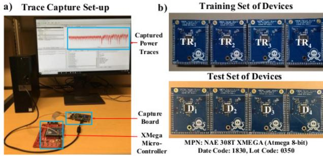
**Figure 2: (a) Trace Capture Set-up using the Chipwhisperer platform. (b) Traces are captured from multiple Atmega microcontroller devices ( $TR_{1-4}$ ) for training a deep neural network (DNN) so that the model is able to generalize to any other target device ( $D_{1-4}$ ).**
