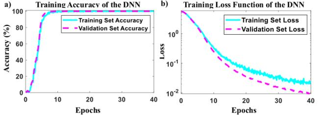
Figure 5: (a) Training and Validation Accuracy of the DNN reaches  $\sim 100\%$  within 25 epochs and does not show any overfitting. (b) Loss function of the DNN for both the training/validation sets. Note that training and validation have been performed with data from all the 4 devices ( $TR_{1-4}$ ).
