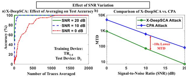
**Figure 11: (a) Number of traces (averaged) required for a successful X-DeepSCA attack (with > 99.9% accuracy) in different SNR scenarios. For SNR=20dB, averaging with less than 10 traces is sufficient to achieve > 99.9% accuracy, while it requires ~ 100 traces for SNR=10dB, and ~ 1000 traces to be averaged over to achieve the 99.9% accuracy. (b) Comparison of the X-DeepSCA attack with traditional CPA attack shows a lower MTD for X-DeepSCA compared to CPA for all SNRs.**
