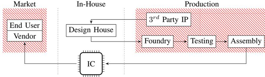
Figure 1: Simplified view on an exemplary, outsourced design fabrication process. Every entity hatched red is untrusted and can potentially be malicious.
