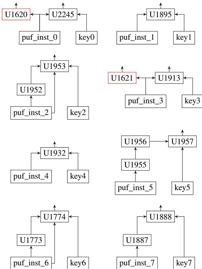
Figure 13: Connectivity of the PUF-related gates in the first variant of the CLIP netlist.
