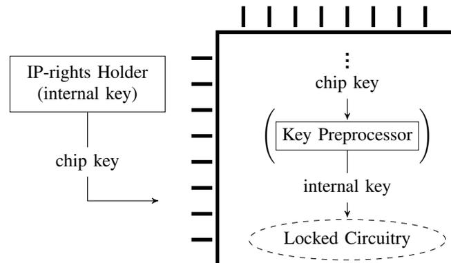
Figure 4: Visualization of the relation between the different keys and elements in logic locking. Note that the key preprocessor is optional.
