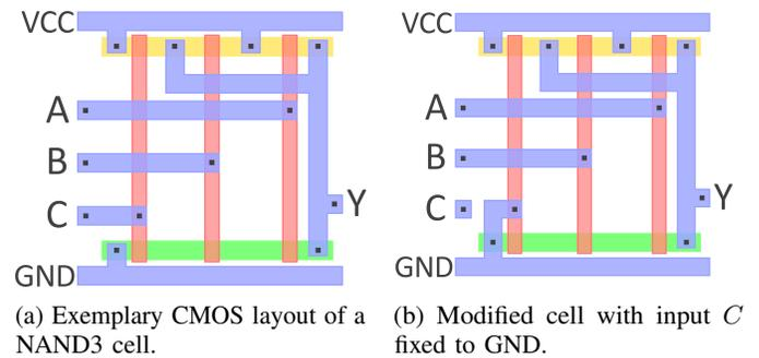
Figure 9: Application of a mask modification attack. Wire spacings and thickness have been adjusted to improve readability. The wire on input  $C$  was cut and directly connected to GND.
