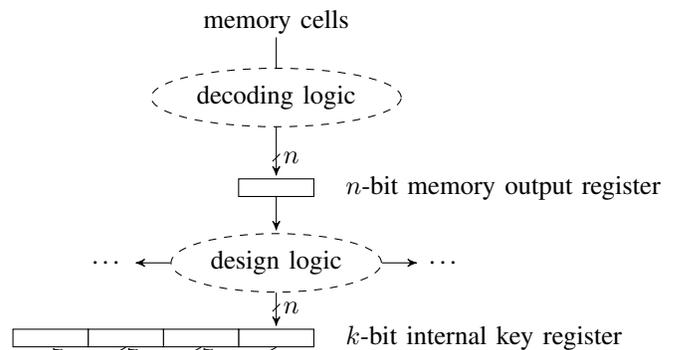
Figure 7: Simplified illustration of the data path from an  $n$ -bit memory interface to a  $k$ -bit key register, where  $k > n$ .
