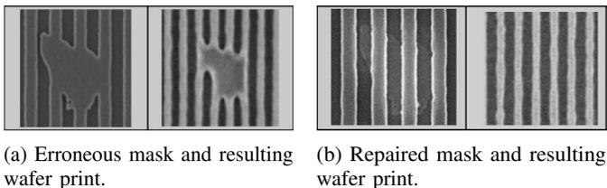
Figure 6: Examples of mask repair [55].
