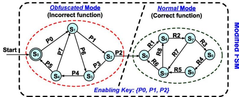
Figure 3: An example of sequential logic locking with HARPOON as depicted in [10]. The locking circuitry facilitates the dummy states on the left while only the correct state sequence leads to the original FSM on the right.
