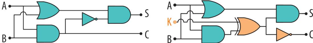
Figure 2: An example of combinational logic locking with EPIC as depicted in [5]. Left is the original design and right the locked result.
