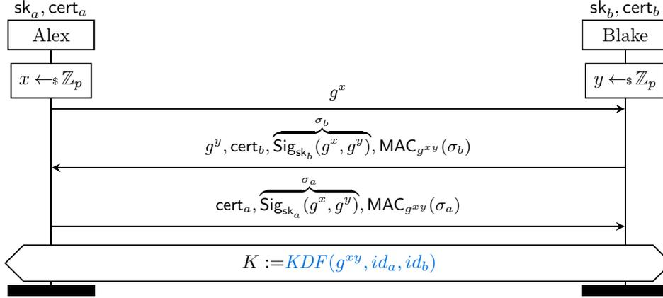
Figure 6: Sketch of STS-KDF [26], which patches STS-MAC by including the identities of the communicating parties in the KDF.
