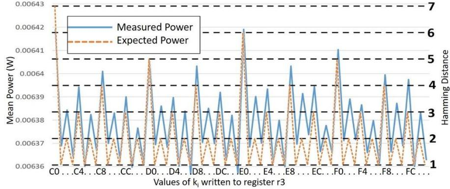
Fig. 5. Correlation of corrected power measurements of `lds` instruction (solid) to Hamming Distances  $HD(r_3', r_3)$  (dashed) at 1 MHz clock frequency. Values of  $k_i$  written to  $r_3$  by `lds r1, r3` are shown on the x-axis, where previous contents of  $r_3$  ( $r_3'$ ) are computed as  $r_3' = r_3 - 1$ .
