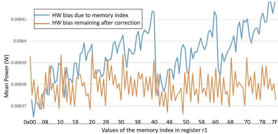
Fig. 6. Power measurements for `lds r1, r3` for `r3` operands with zero Hamming Distance. Hamming Weight (HW) bias due to memory index in `r1` shown in top line, and attempted removal of HW bias shown in bottom line.
