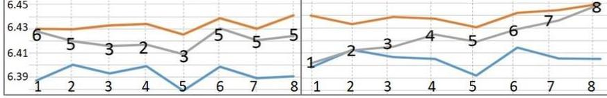
Fig. 4. Measured power of minimum HW reference (bottom), maximum HW reference (top), and test vector (TV) with actual HW of each byte (middle); TV1 shown at left, and TV2 shown at right. Power in mW is shown on y-axis.
