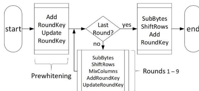
Fig. 2. AES Encryption with Iterative Round Structure
