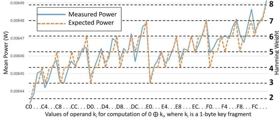
Fig. 3. Correlation of measured power at 1 MHz clock frequency (solid) to Hamming Weight (HW) of operand (dashed) for `xor` instruction. Mean power depicted on left (in Watts); HW of operand is on right.
