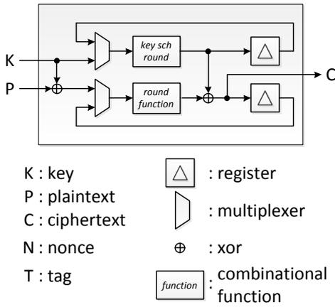
Fig. 1. Generic block diagram of the block cipher cores
