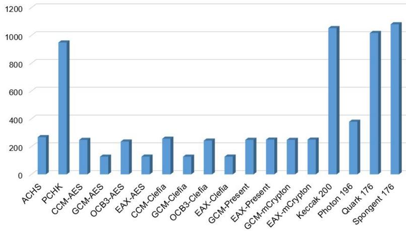
**Fig. 9.** Speed results (MHz)
