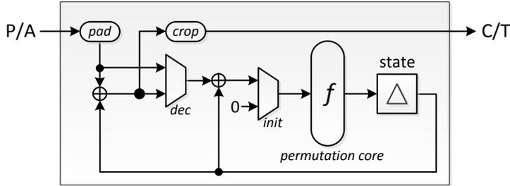
Fig. 7. Block diagram of the permutation-based authentication encryption scheme wrapper
