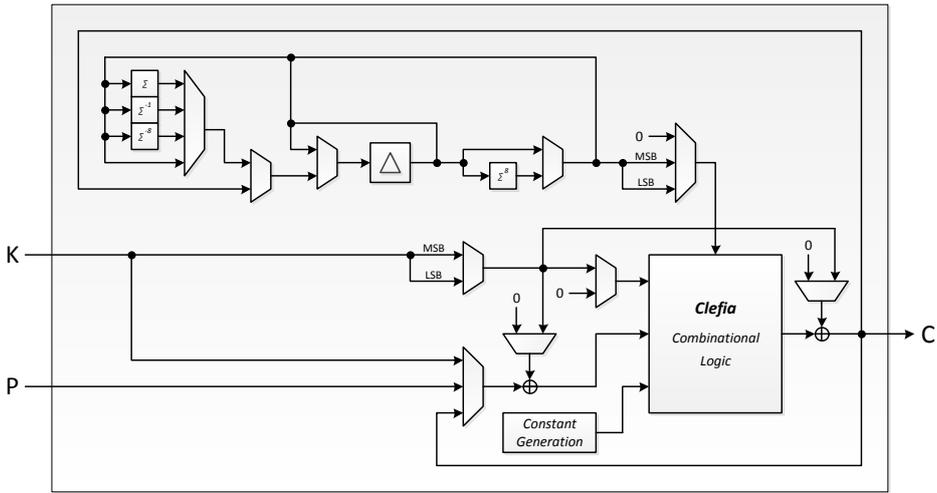
Fig. 2. Detailed block diagram of the Clefia block cipher core
