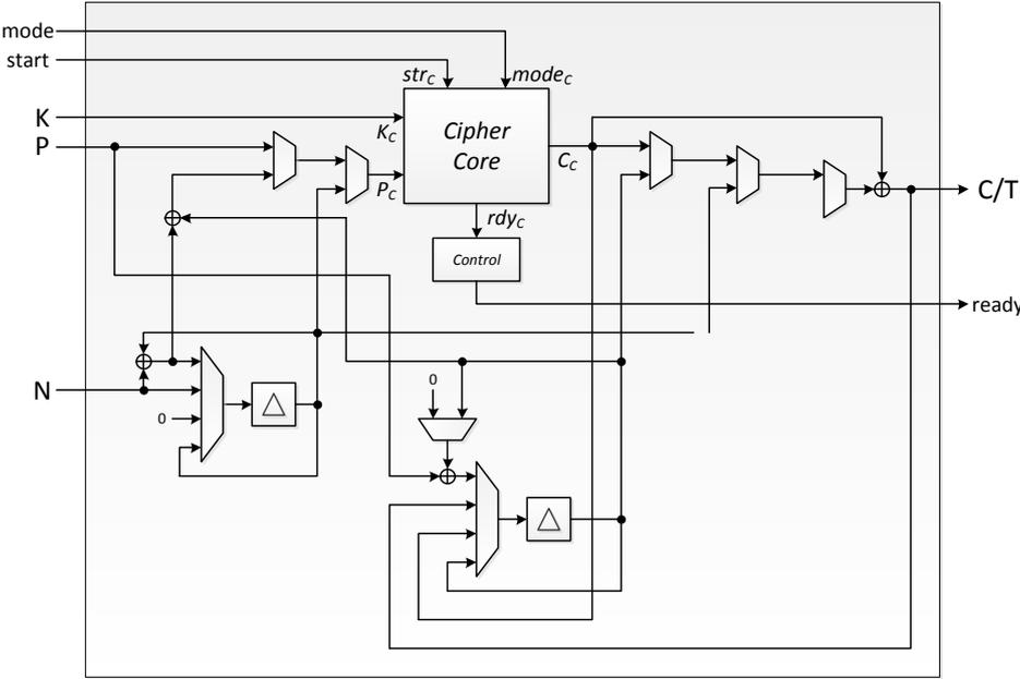
Fig. 5. Block diagram of the OCB3 authentication encryption scheme wrapper
