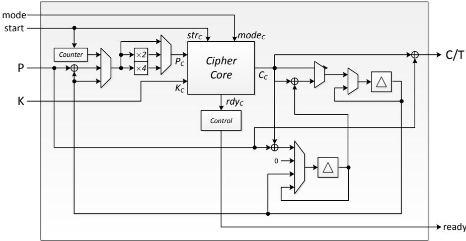
Fig. 6. Block diagram of the EAX authentication encryption scheme wrapper
