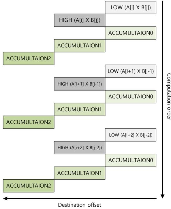
Fig. 3: Part of column-wise multiplication for ARMv8
