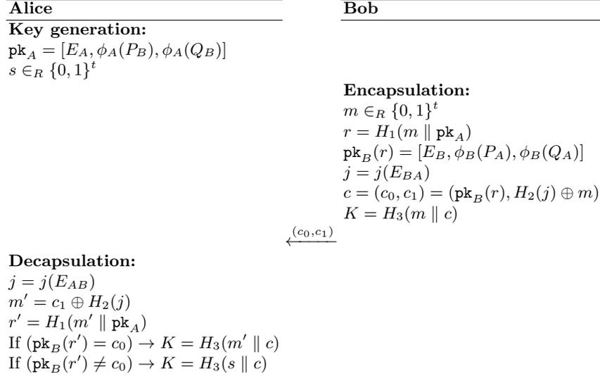
Fig. 2: SIKE mechanism.
