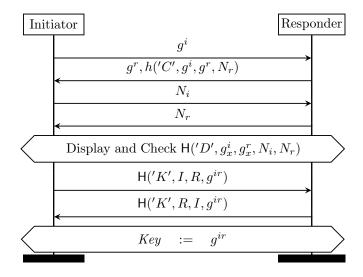
Figure 2: Bluetooth's Simple Secure Pairing Handshake
