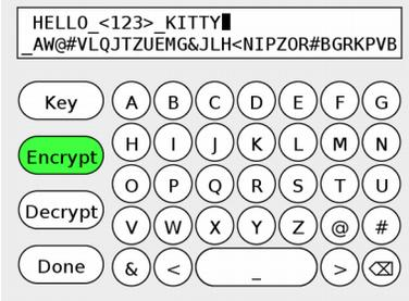
Once the plaintext is complete, Alex taps the “Done” button. The appliance computes the message authentication tag, which appears at the end of the ciphertext. (The E2K application does not support additional authenticated data; the header is always empty.) Alex can scroll the display by swiping it left or right. Alex types the ciphertext message into an online computer for transmission to Blake.
