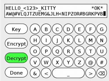
After typing the entire ciphertext including the tag, Blake taps the “Done” button. The appliance authenticates the message. If the authentication succeeds, the display shows “OK” along with the plaintext.
