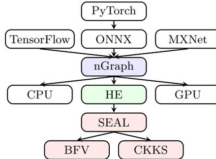
Fig. 1: Overview of the nGraph-HE software stack. nGraph-HE currently supports the SEAL encryption library [36], and the underlying cryptosystems BFV [5] and CKKS [18], and it can be extended to support additional cryptosystems.
