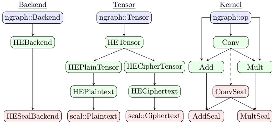
Fig. 4: Visualization of nGraph-HE architecture. Objects with the same color interact. The dotted line from `Conv` to `ConvSeal` indicates optional overriding of the default `Conv` implementation.
