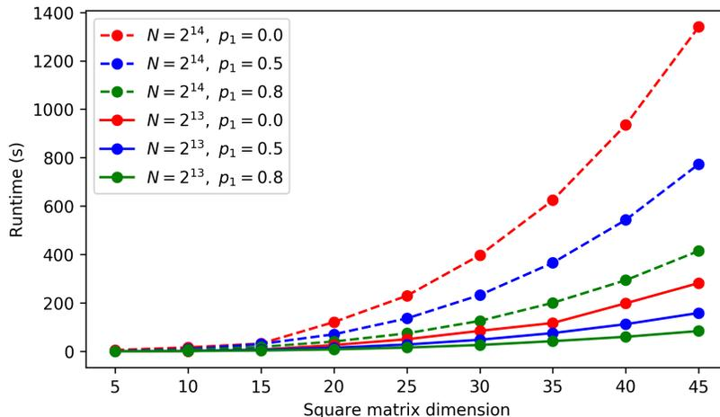
Fig. 5: Single-threaded runtime on GEMM operations as a function of matrix size, polynomial modulus, and sparsity.
