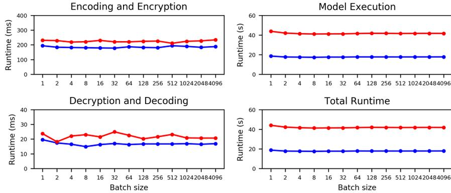
Fig. 6: Runtimes on pre-compiled CryptoNets network with HE-SIMD packing for different batch sizes, for  $N = 2^{13}$  (—) and  $N = 2^{14}$  (—).
