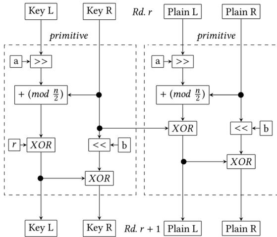
Figure 2. A single round  $r$  of the SPECK cipher for  $n$ -bit input,  $a=8$  and  $b=3$  in the original NSA publication [2]
