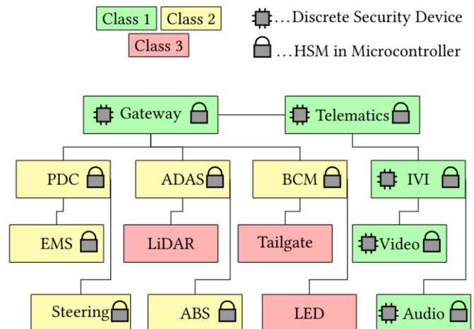
Figure 1. Hardware security features in selected control units arranged in a modern topology
