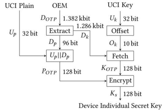
Figure 3. Applied example of the key derivation scheme
