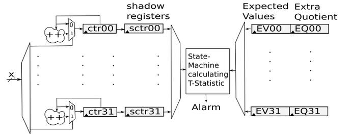
Fig. 3. Hardware architecture of the proposed expensive countermeasure.
