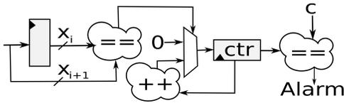
Fig. 1. Hardware architecture of the proposed low cost countermeasure.
