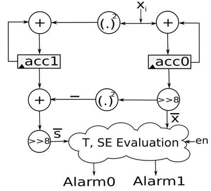
Fig. 2. Hardware architecture of the proposed standard countermeasure.
