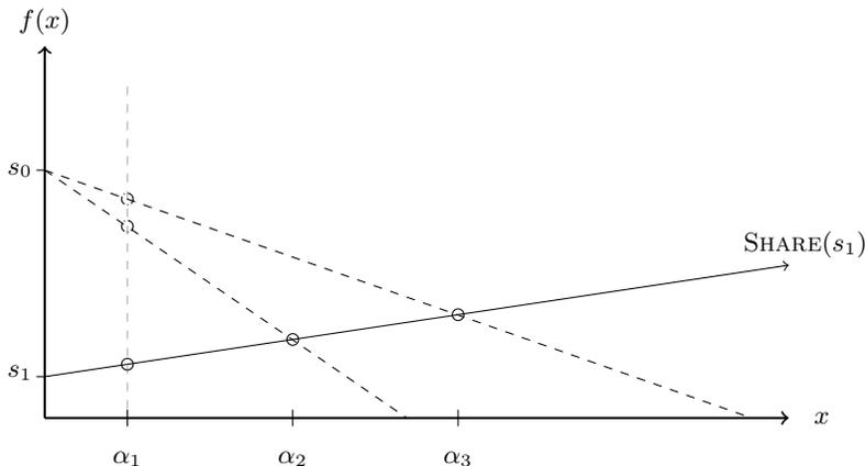
**Fig. 2.** Illustration of our efficient attack on 2-out-of- $n$  Shamir secret sharing. The secret shared value is  $s_1$  and the solid line represents the linear function that was used during the secret sharing. The dashed lines depict the linear functions that are interpolated from the shares under the assumption that the secret shared value is  $s_0$ . Two distinct incorrect points at  $x = \alpha_1$  are extrapolated.
