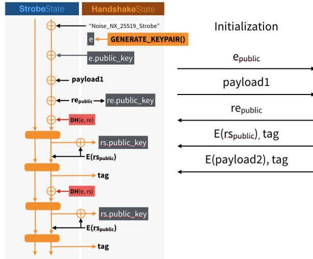
Figure 10: The Disco NX handshake pattern view from the inside. Absorption has been simplified: if the input is larger than the rate, the state needs to be permuted in between smaller absorptions.
