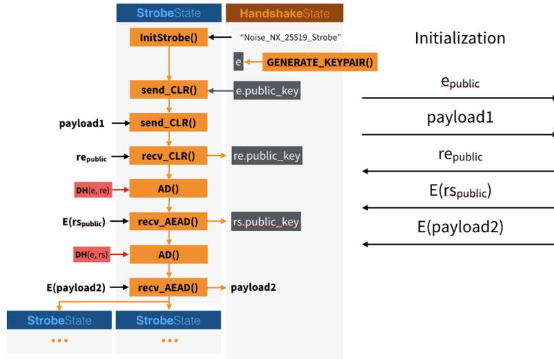
Figure 9: The NX pattern within Disco. Both the CipherState and SymmetricState have been removed in favor of a unique and simple StrobeState.
