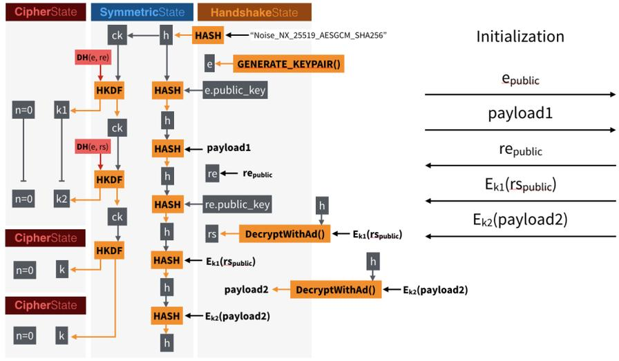
Figure 8: A simplified representation of the *NX* handshake pattern of the Noise protocol framework. As can be seen, three different states are maintained by a peer, one used to store asymmetric keys, one used to store the running hash and the chaining key, one used to store derived keys used for encryption.
