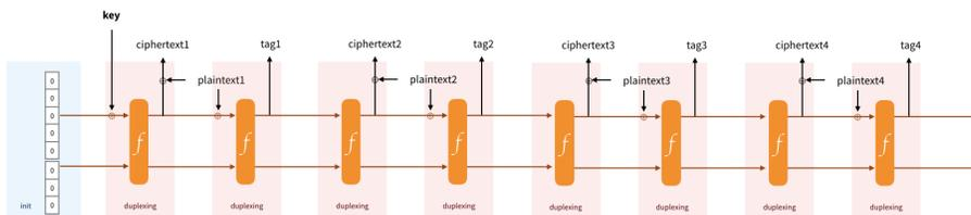
Figure 4: A session built from the duplex construction. Each tag not only authenticates the previous encryption, but any operation that has happened prior to it.
