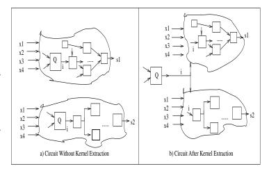
Fig. 2. Circuit of s1 and s2 with and without Kernel Extraction
