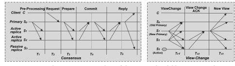
Figure 3: The consensus procedure of the proposed scalable BFT protocol.
