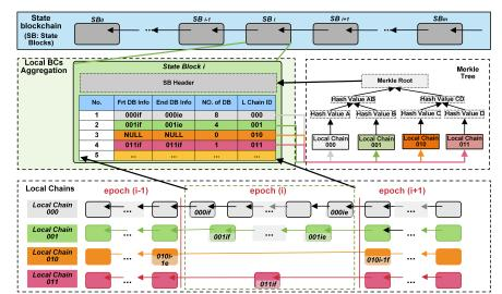
Figure 2: Blockchain design in SMChain. Each block epoch has only one state block but multiple data blocks.
