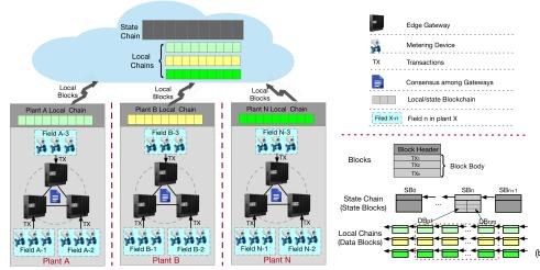
Figure 1: (a) An overview of the SMChain architecture with three components: local metering networks, local chains stored in the plants, and the state chain stored in the cloud; (b) The conceptual chain structure between local chains and the state chain.
