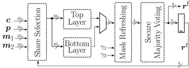
Fig. 7. Application of our construction on Interpose PUF.
